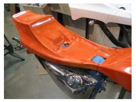
Ideally a floating tank and a locked down tail will result in a kiss fit between tank and tail.
