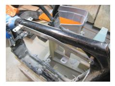
Little hands on the slotted mount brackets catch the tank studs
