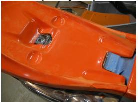
The tail mounts simply. The front tab (blue painters tape) secures the tail front. do Often you'll have to bend this tab up (for more clearance) or down to tighten the clamping power on the tail front. Notice the dropped area with the frame poking through. That is for a ½-20 screw-the only fastener that holds the tail in place
